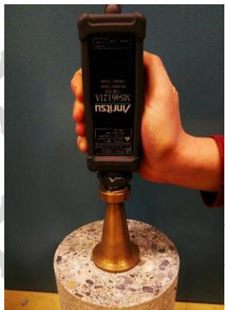
Acquisition of the S11 parameter on the surface of a concrete sample.
