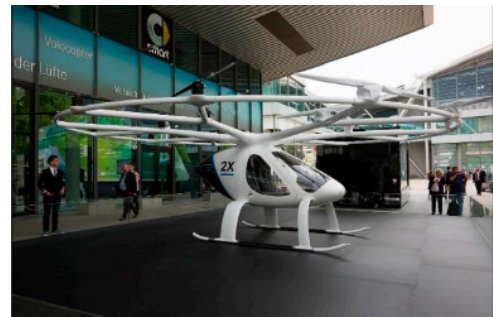
Figure 1 Wingless Multirotor E-VTOL: Volocopter 2X [4]
