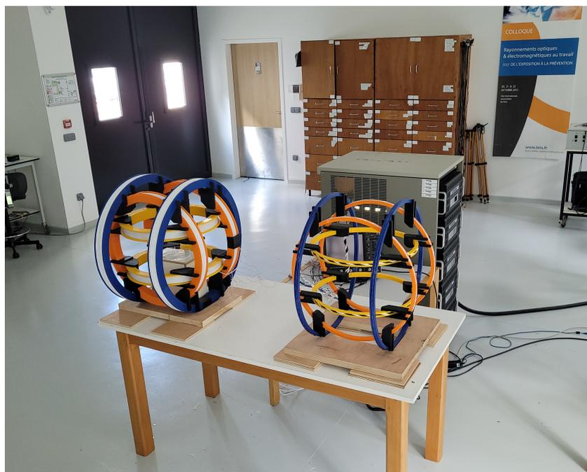
Figure 1: Helmholtz coils at the INRS electromagnetism laboratory.
