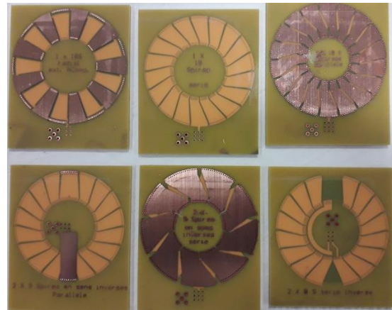
Figure 2 PCB embedding Inductor
